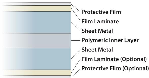
surfaces where sound damping is desirable and where stringent demands are placed on visual expression and function. The product is available with both galvanised sheet metal and aluminium as the base material. It can be delivered with various types of inner layer in order to provide different properties in response to different needs.
